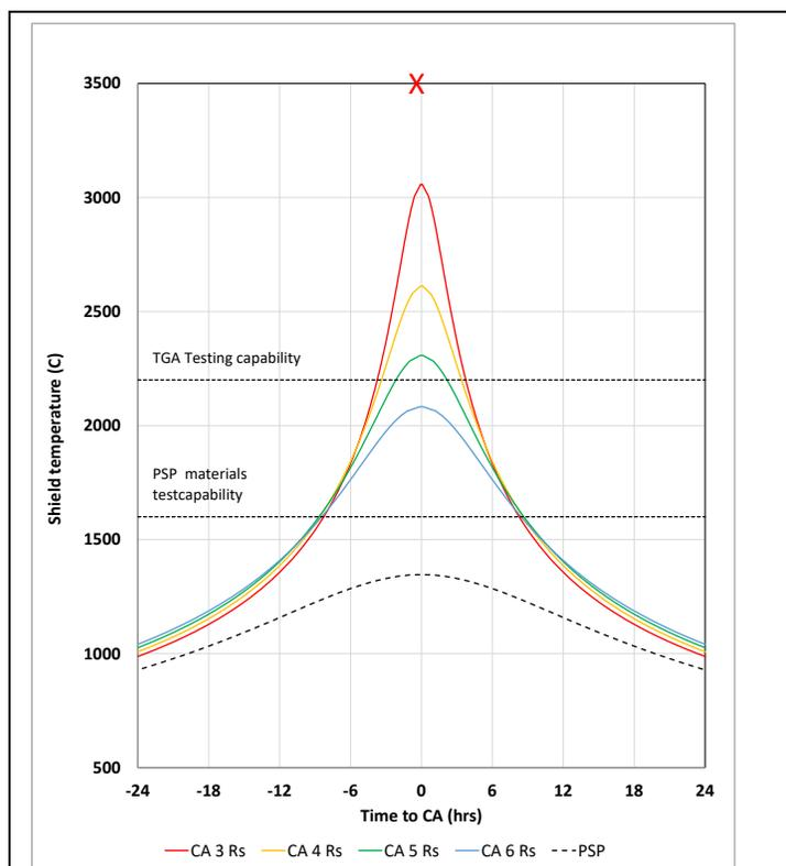
Figure 1. Near-Sun pass shield temperature profiles and testing capabilities
